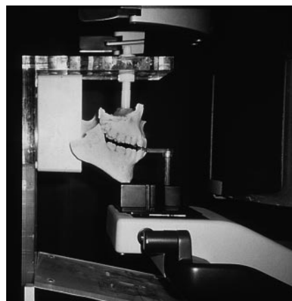
Fig.4 Resected jaws fixed in the beam path of the OPG modified by the spine phantom and the soft tissue filter
